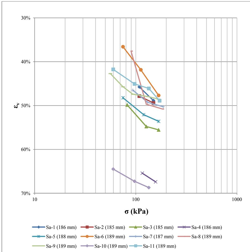
Figure 3. Settlement curves. Vertical strain against applied pressure.
