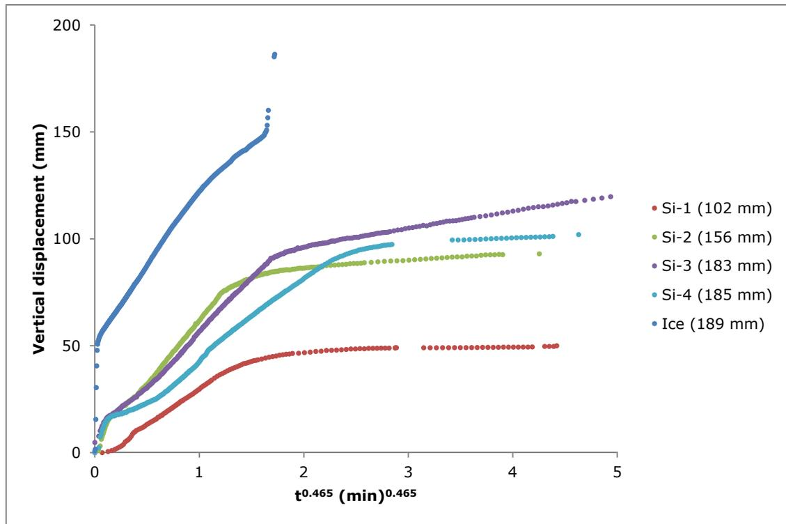
Figure 2. Single load thaw consolidation test on silty frozen soil. Vertical displacement against time at 0.465 power.
