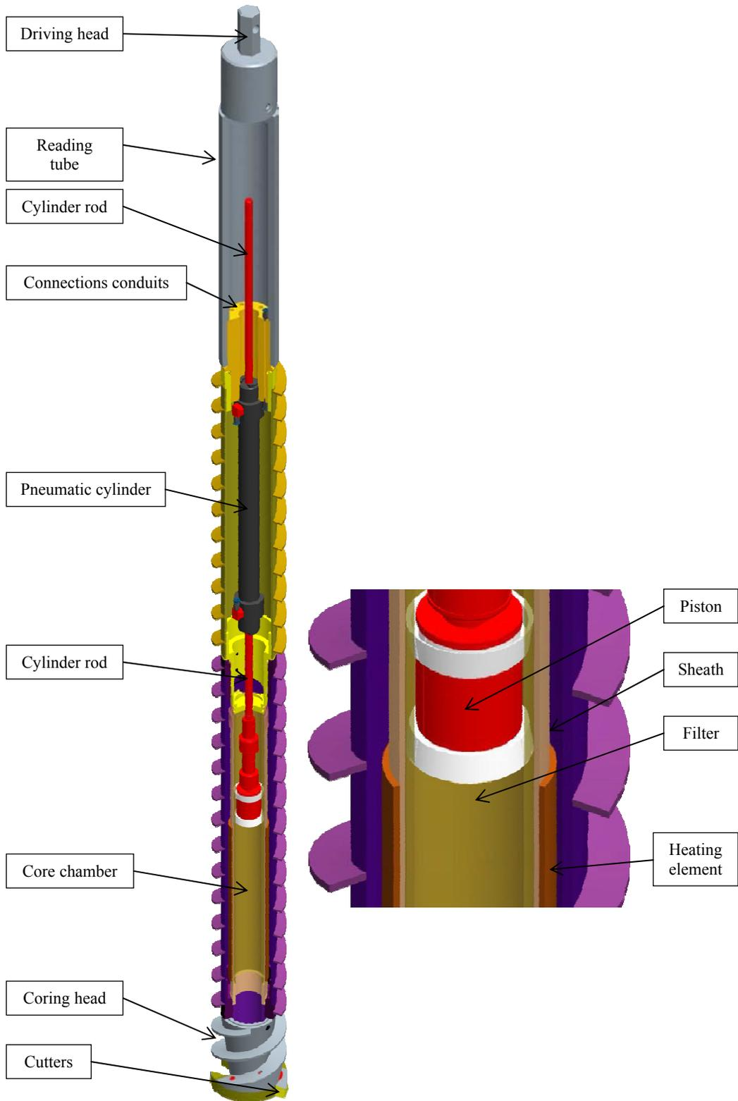
Figure 1. Core barrel view.
