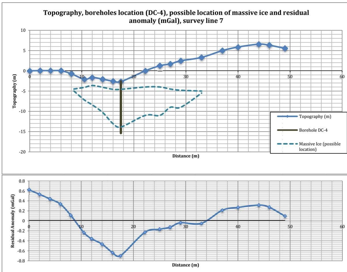
Figure 6. Microgravimetric survey line 7 with borehole localisation (DC-4) and residual anomaly.
