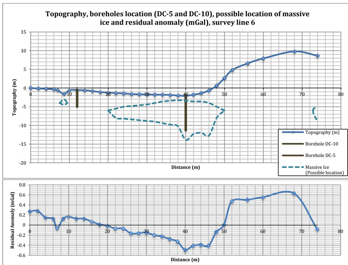
Figure 5. Microgravimetric survey line 6 with boreholes localisation (DC-5 and DC-10) and residual anomaly.
