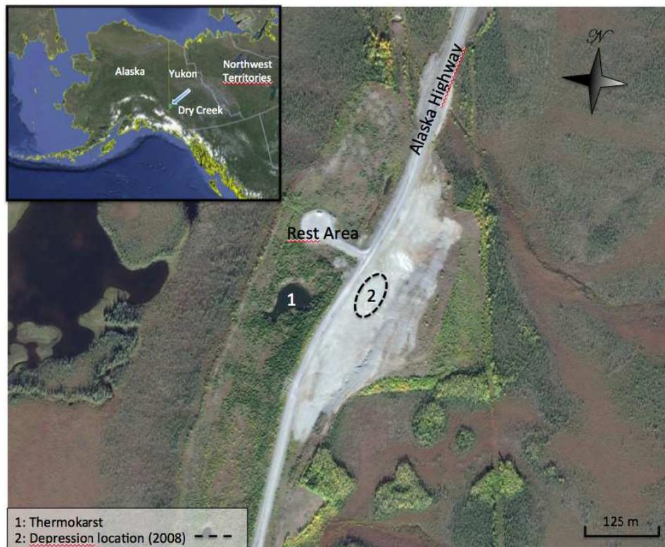
Figure 1. Study site location: Dry Creek rest area, south-western Yukon. 1) Thermokarst lake; 2) former gravel borrow pit where large depressions and sinkholes were observed over the years (1994-2014). The zone left of the highway has also been stripped of its vegetation and surface gravel cover in the past but is now colonized by vegetation (source: Google Earth, 2015).
