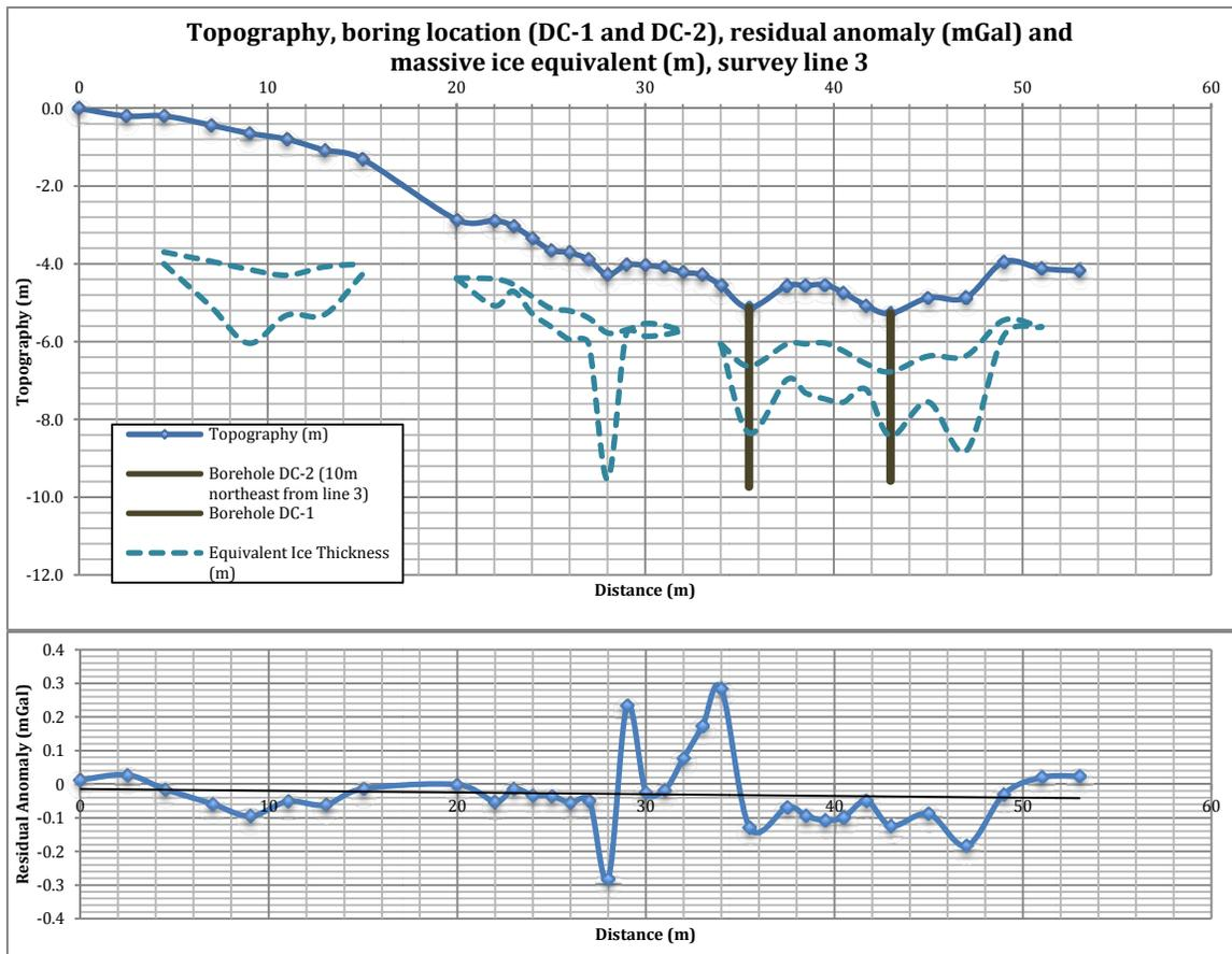
Figure 4. Microgravimetric survey line 3 with boreholes localisation (DC-1 and DC-2) and residual anomaly.
