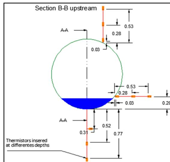
Figure 2 : Instrumentation at Border Culvert site
