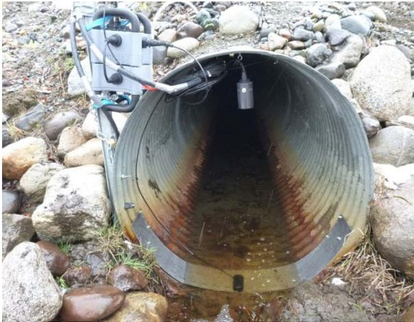
Figure 4 : Flow measurement system in the second year. Water velocity was measured by the lower sensor, shown submerged, and water height by the upper sensor.
