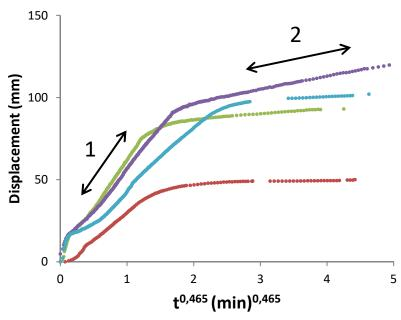
Displacement as a function of time (McKinley, 1961) Phase 1: Thawing and draining of excess ice (20-40 min.)
