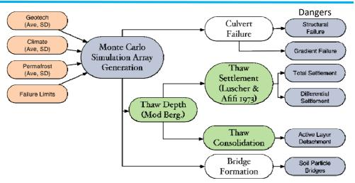
Hazard Calculation Process: Inputs (orange) of stochastic variables for average (Ave) and standard deviation (SD), calculations (green) and hazard calculations from the limit state functions (blue).
