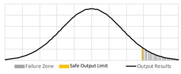
random variables considered in the analysis are randomly selected from defined probability density functions. Calculating the limit state function result with the randomly varied input properties many times (simulations) results in the statistical variation of the limit state function. The hazard is calculated from the
