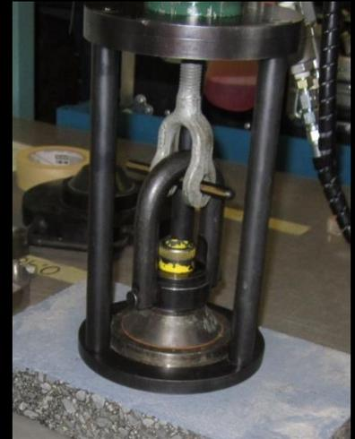
Test de tension direct – LC 25-010
